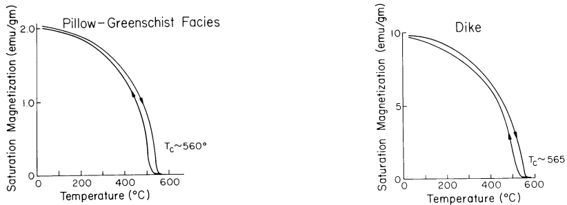
Fig. 1. Thermomagnetic curve for typical pillow basalt and dike samples for the three ophiolite complexes. The experiments were done in vacuum ( < 5 \times 10^{-6} torr) and an applied field of 2.5 \times 10^3 Oe.
