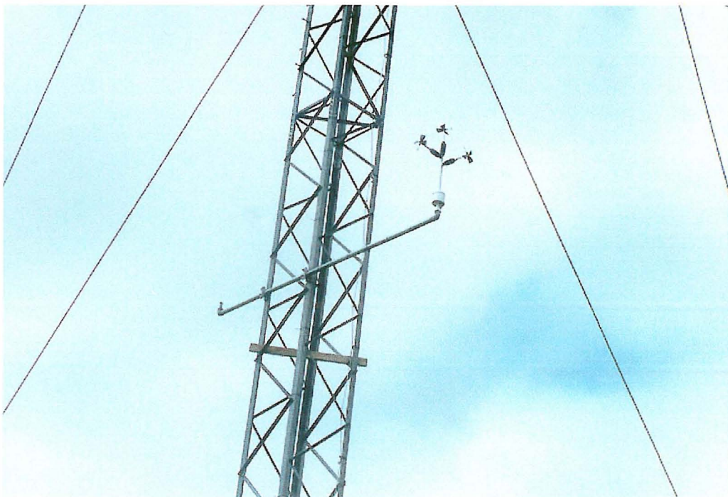
Fig. 5. The lower of the two Gill UVW anemometers at Leirur. Photo: Hreinn Hjartarson, 1993.
