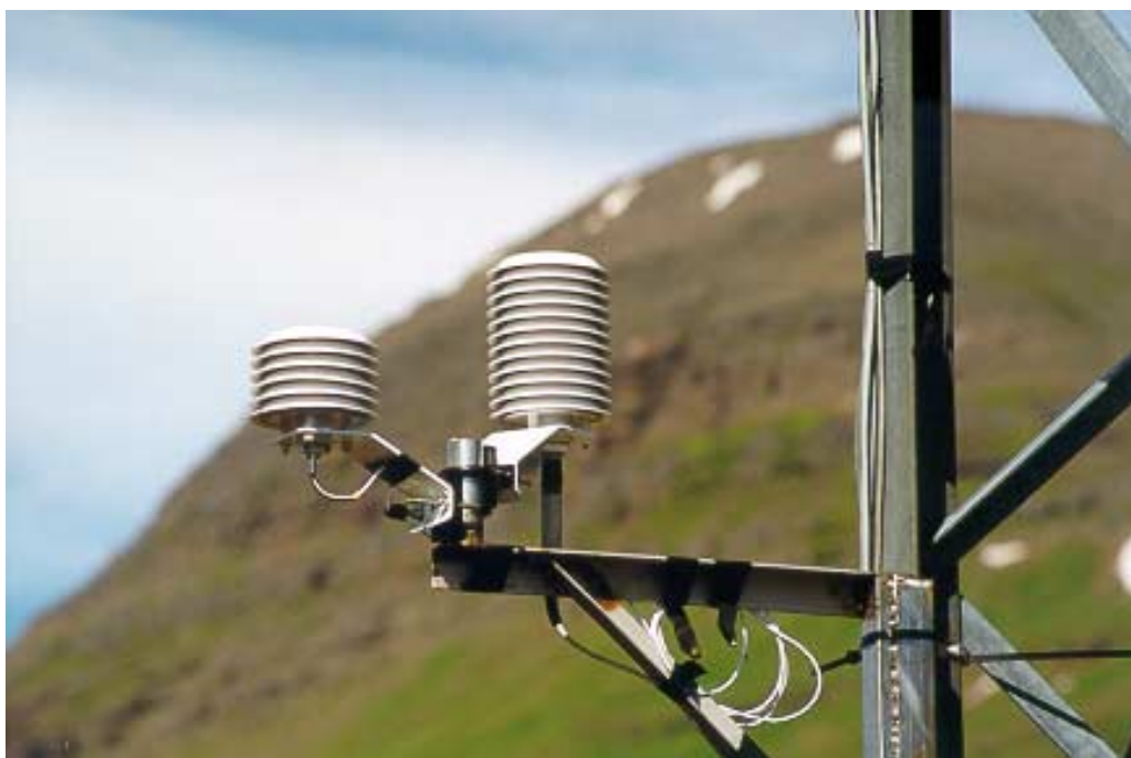
Fig. 3. Thermometer and hygrometer at 3.0 m above the ground. Photo: Flosi Hrafn Sigurðsson, 1999.
