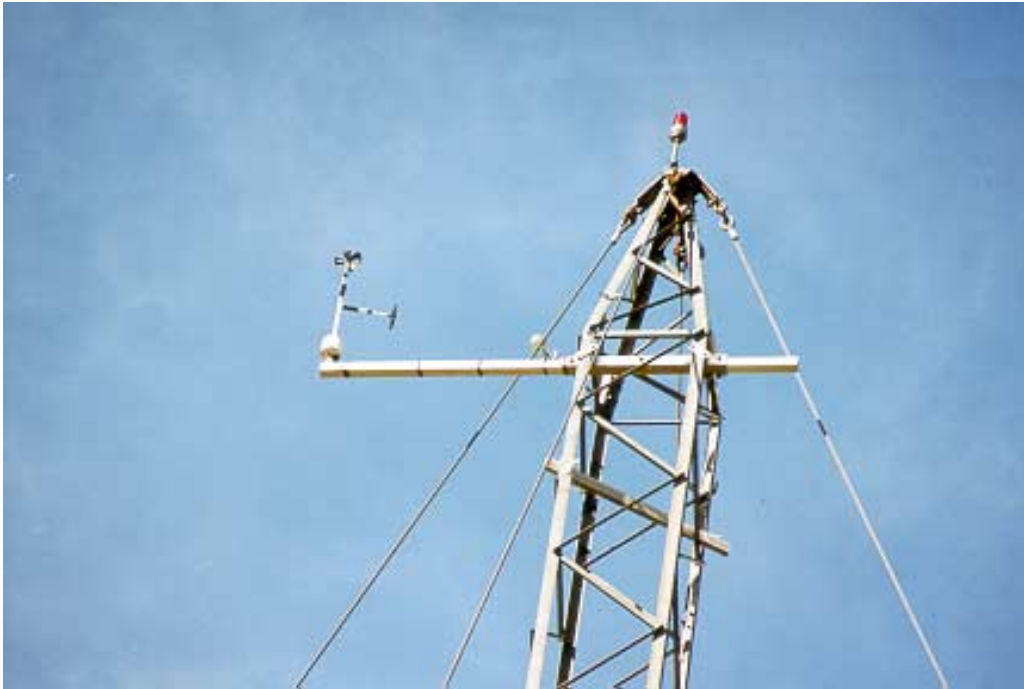
Fig. 4. Gill UVW anemometer and thermometer near the top of the mast. Photo: Flosi Hrafn Sigurðsson, 1999.
