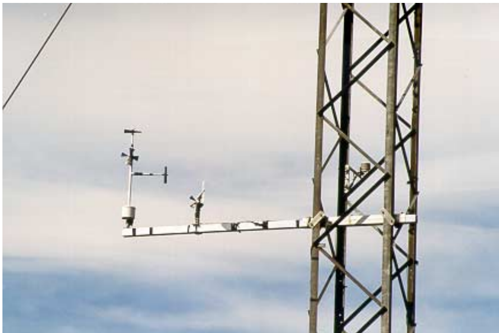
Fig. 5. Anemometers and thermometer at 10.3 – 10.8 m above the ground. Photo: Flosi Hrafn Sigurðsson, 1999.
