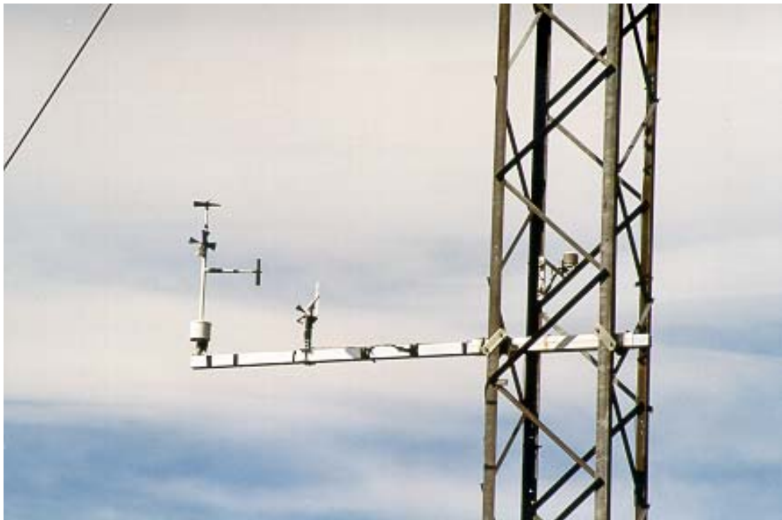
Fig. 3. Anemometers and thermometer at 10.3 - 10.8 m above the ground at Sómastaðagerði. Photo: Flosi Hrafn Sigurðsson, 1999.
