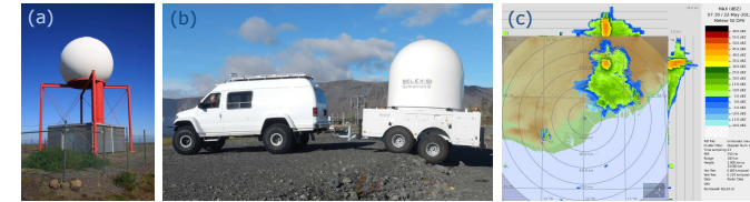
(a) The Keflavík C-band weather radar, (b) Huginn mobile radar, (c) A sample radar reflectivity plot during the Grímsvötn 2011 eruption measured by the Italian mobile radar. Photos Pörður Arason and Geirfinnur S. Sigurðsson.
