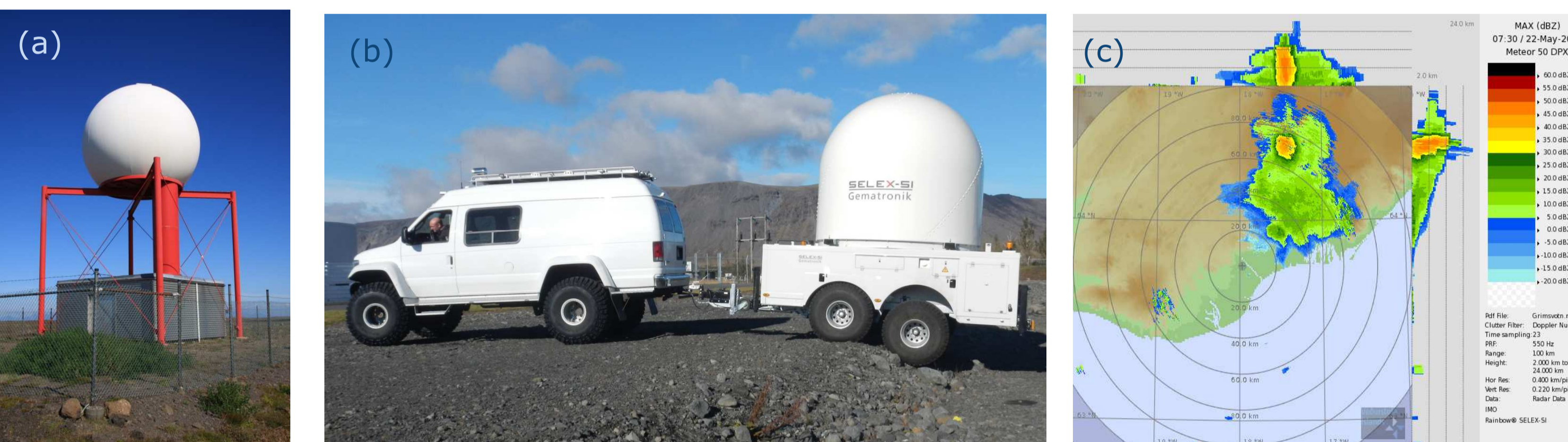
(a) The Keflavík C-band weather radar, (b) Huginn mobile X-band radar, (c) A sample radar reflectivity plot during the Grímsvötn 2011 eruption measured by a mobile radar on loan from the Italian Civil Protection Authorities (Selex Meteor 50DX). Photos Þórður Arason and Geirfinnur S. Sigurðsson.
