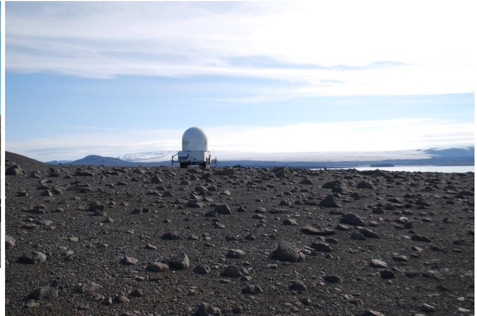
Mobile radar installed with clear view over Bárðarbunga before the eruption. Photo Þorgils Ingvarsson 22 August 2014
