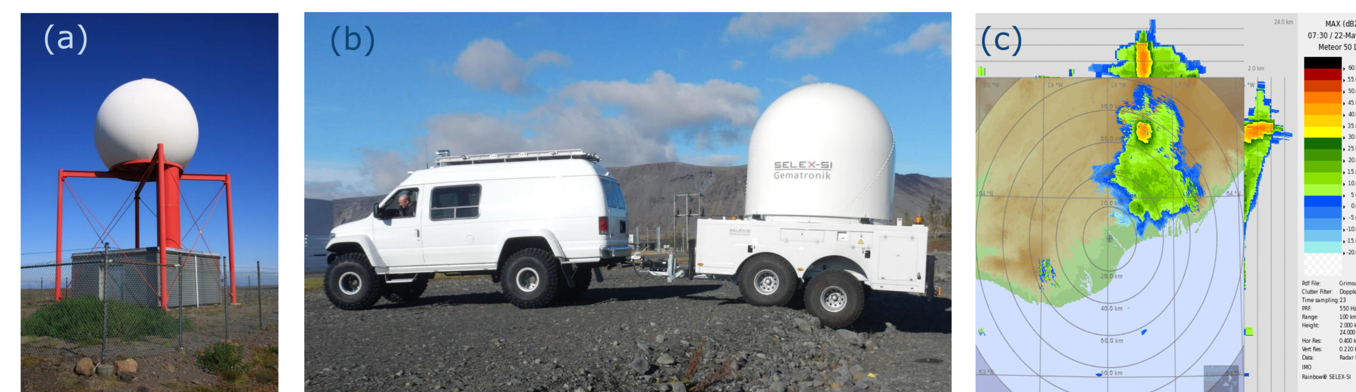
Figure 4. Icelandic Radar System. (a) The Keflavík C-band weather radar, (b) Huginn mobile X-band radar, (c) Radar reflectivity during the Grímsvötn 2011 eruption measured by a mobile radar. Photos Pórður Arason and Geirfinnur S. Sigurðsson.
