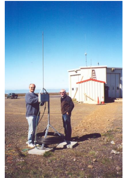
Technicians from UK Met Office set up an ATD-sferics out-station in Keflavík, SW-Iceland. Photo Þórður Arason 4 July 2002.
