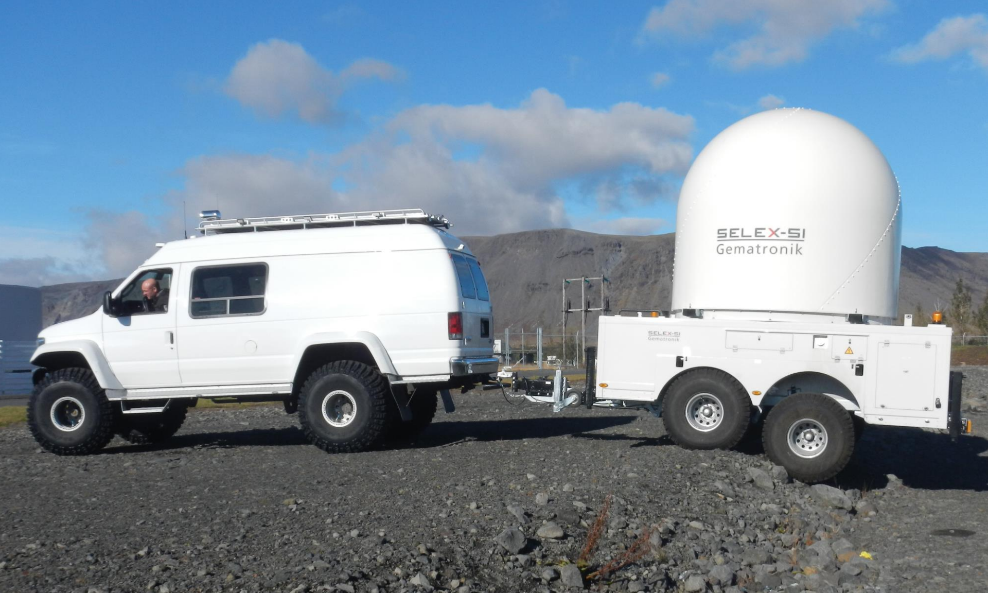
Specially adapted truck to take mobile radar off road. Photo Geirfinnur S. Sigurðsson 25 September 2012
