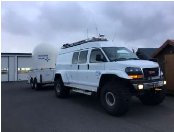
Specially adapted truck to take mobile radar off road. Photo Hermann Arngrímsson 25 September 2016
