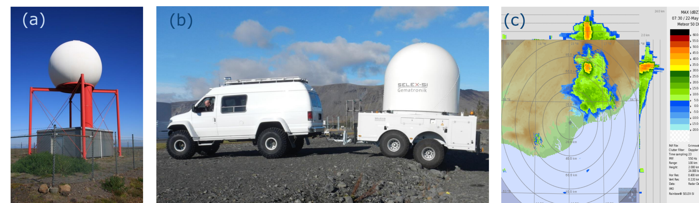
Figure 4. Icelandic Radar System. (a) The Keflavík C-band weather radar, (b) Huginn mobile X-band radar, (c) Radar reflectivity during the Grímsvötn 2011 eruption measured by a mobile radar. Photos Þórður Arason and Geirfinnur S. Sigurðsson.
