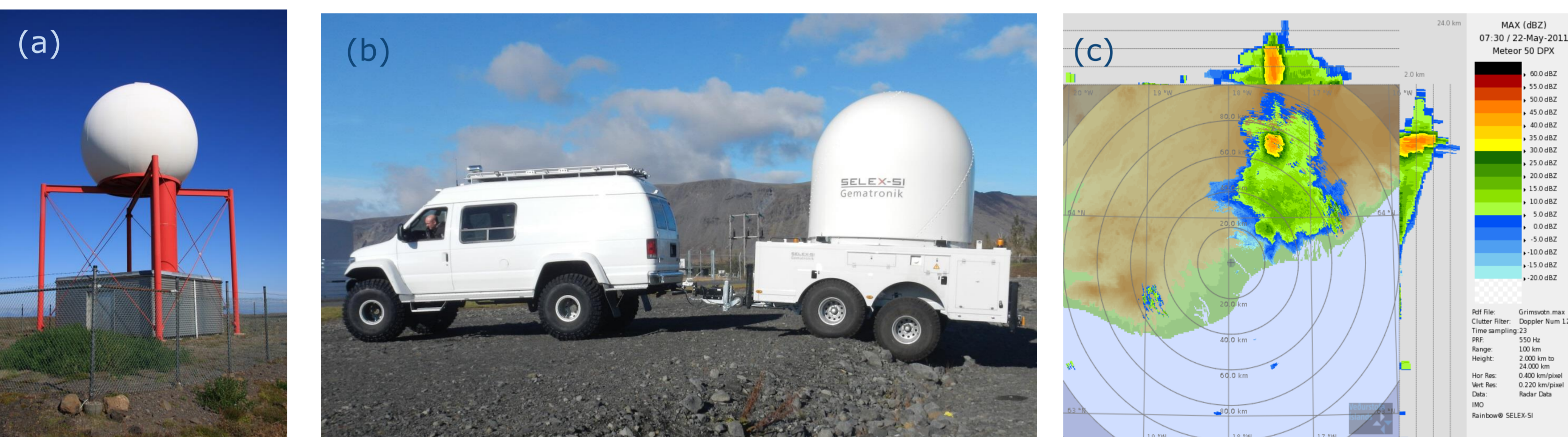
(a) The Keflavík C-band weather radar, (b) Huginn mobile X-band radar, (c) A sample radar reflectivity plot during the Grímsvötn 2011 eruption measured by a mobile radar on loan from the Italian Civil Protection Authorities (Selex Meteor 50DX). Photos Þórður Arason and Geirfinnur S. Sigurðsson.
