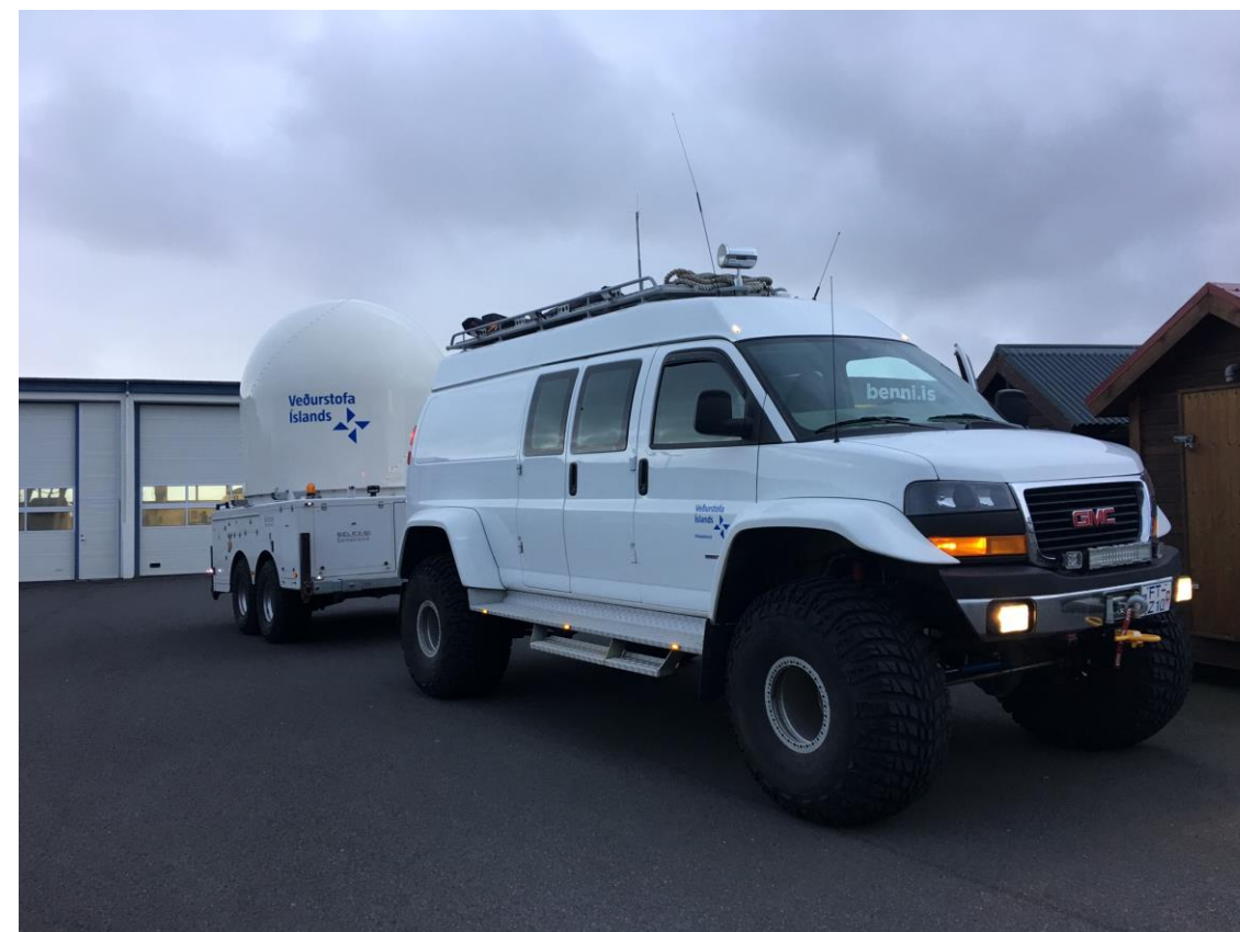
Specially adapted truck to take mobile radar off road. Photo Hermann Arngrímsson 20 October 2016.
