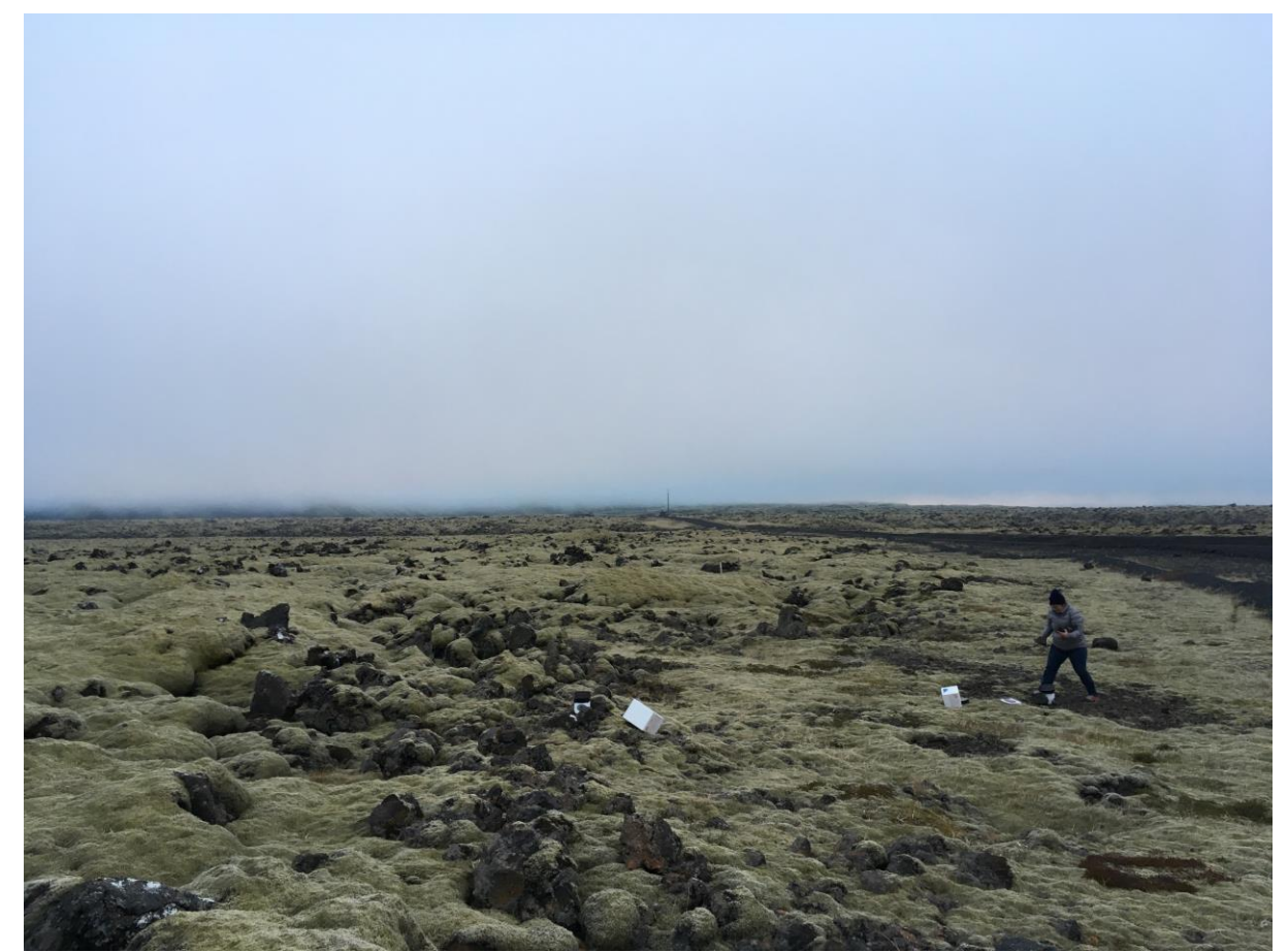
At each location, two rain buckets were placed, about 10-30 m apart, at ground level
