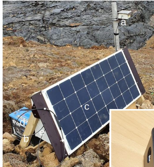
RaspberryPi Picam based system
